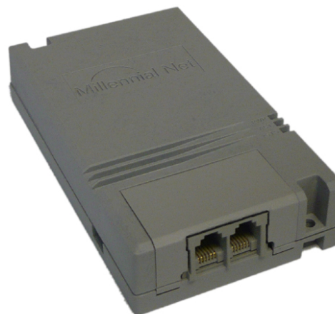
The Wi-Pulse supports two pulse outputs with RJ11 connectors for easy installation. Additional IO interfacing is also possible.
