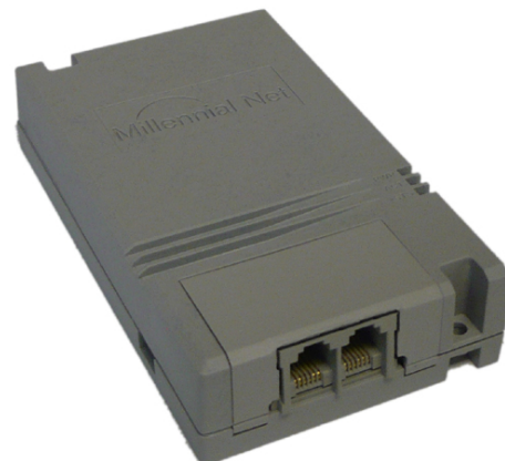
The Millennial Net Wi-IO is a general purpose node featuring two RJ11 connectors with six conductors each, to interface a variety of sensors and actuators to a wireless mesh sensor network.
